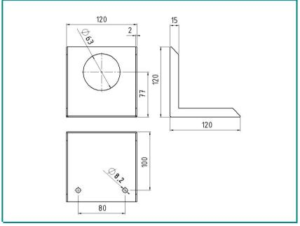
The wall mounting bracket with the corresponding housing nut assures the secure mounting of the pressure regulator PHR.
