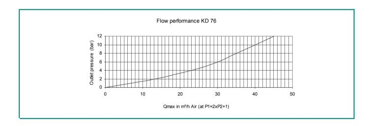
The cylinder regulator KD 76 reduces the pressure of compressed gases as well as liquid gases. The KD 76 finds use where a uniform outlet pressure is guaranteed without constant readjustment.
