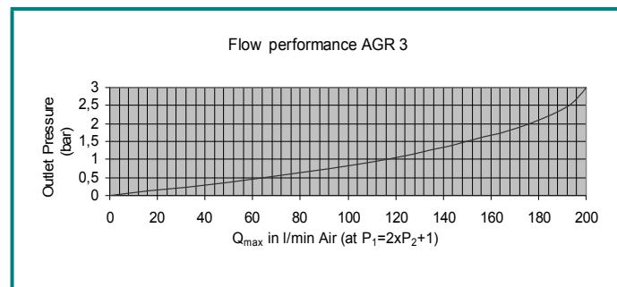
The regulator AGR 2/3 is manufactured in steel C45 or stainless steel 1.4305 for the use in aggressive medium. The gasket and diaphragm material are resistant to the corresponding gas type.
